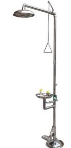
Eye wash shower Foot operated, Body shower Hand operated Suitable to be attached to the ground with its own footplate Shower bowl stainless steel 300 mm All pipes are made of stainless steel
