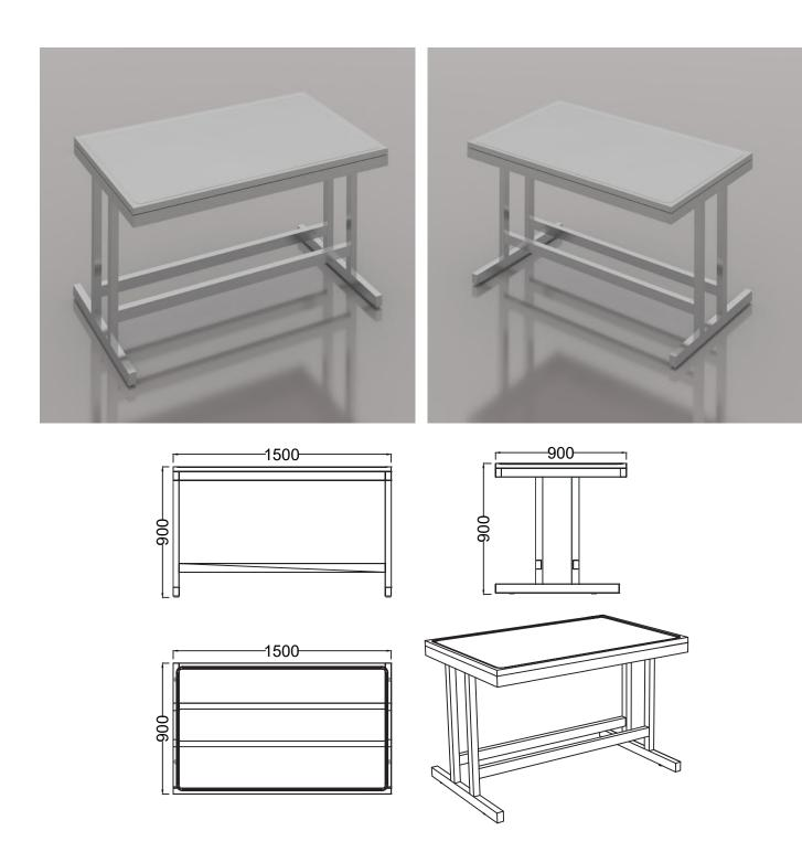
40\*60\*2 Profile Stainless C-Foot and Sleepers 2mm Stainless Steel Working Floor- 33mm Height with Self Cockpit. All screws to be used in stainless products should be stainless
